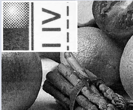
Kyocera: After almost 400,000 pages the perfect quality is reduced. Replacing the developing unit and cleaning the loading mesh improved the quality.
